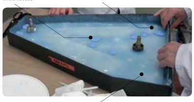
RT Gel: silicone RTV-2 self-adhesive gel for removable adhesion of cured RTV parts
